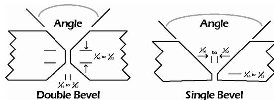
The sections should be separated by a distance of 1/16" to 3/32" to allow the weld metal to flow through the joint without burning the base metal. Sections should never be beveled or chamfered to a knife-edge because the sharp edge will inevitably be burned. An important precautionary measure is to clean the metal adjoining the weld area for a distance of at least 2". This prevents oxides or foreign matter contaminating the weld.
