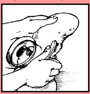
1. Wire brush thoroughly to break up any surface oxide and to remove paint. Grind the damaged edges to a 45° bevel.
